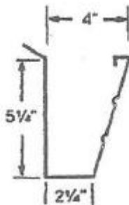
FASCIA GUTTER WITH FLAT, RIBBED FACE
